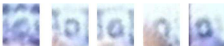
Fig. 10. Low-resolution images of some characters from the iPhone keypad. Can you recognize these characters? Note that at these low resolutions, it is an exceedingly difficult task for humans—let alone OCR engines—to recognize the character corresponding to each image. In the absence of additional information, this is the main reason OCR systems often fail completely when applied to this task. (Answer: reading left to right, C D G O Q).
