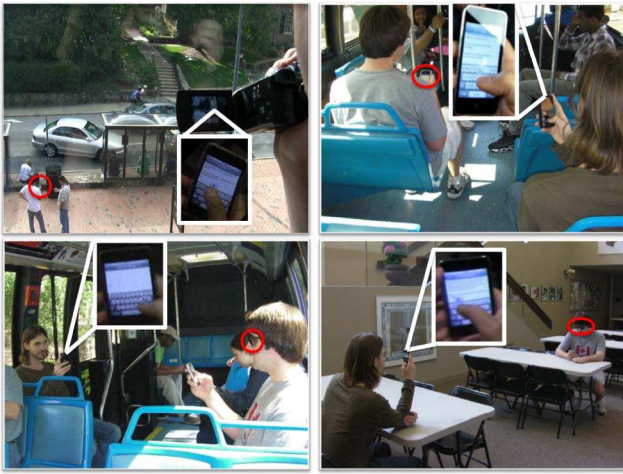
Fig. 1. Example threat scenarios that we investigated. Video was recorded in both indoor and outdoor environments, using various consumer video cameras. Top: shoulder surfing. Bottom: reflection surfing. Observe the key pop-out events in the inset images.
