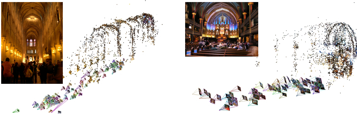
Fig. 16 Two models for different parts of the Notre Dame cathedral interior. The model on the left consists of 118 cameras, 5167 3d points and 28398 2D projections. The model on the right consists of 65 cameras, 6458 3D points and 2D 30609 projections.
