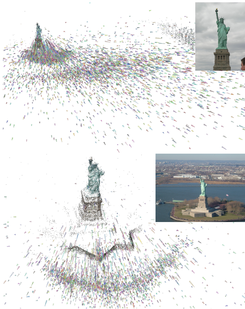
(a) Two views of the Statue of Liberty in New York (9025 cameras, 34234 3D points, 2024119 2D projections).
